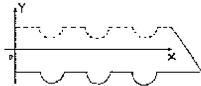
Figure 5-4 Symmetry block element to X axis
